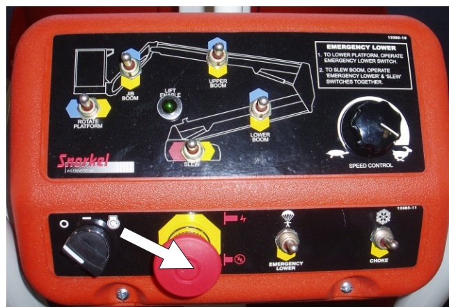
Figure 8.2 - Platform Control Box Emergency Stop Switch Location.
